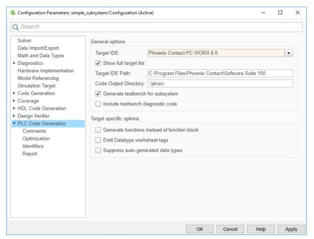
4 On the **PLC Code Generation** pane, select an option from the **Target IDE** list, for example, 3S CoDeSys 2.3.
